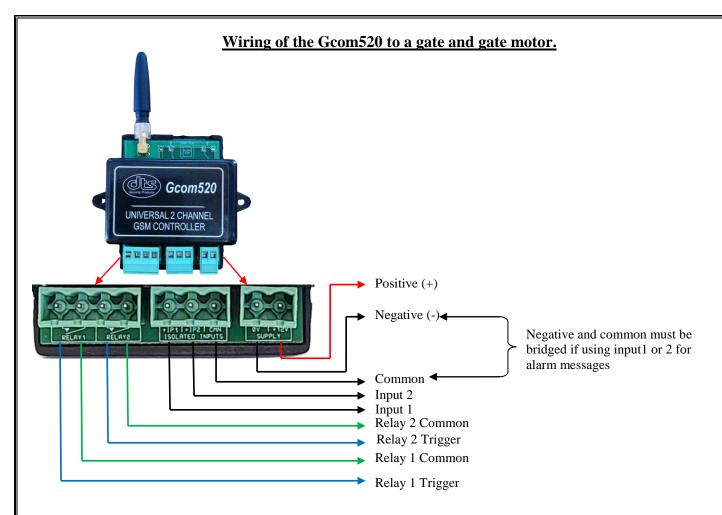
Please note that if the Gcom520 is located or mounted in a metal housing, the existing antenna must be removed and replaced with an external antenna with a SMA-RF connection (Note: when replacing or changing out antenna's, ensure the unit is powered down).
